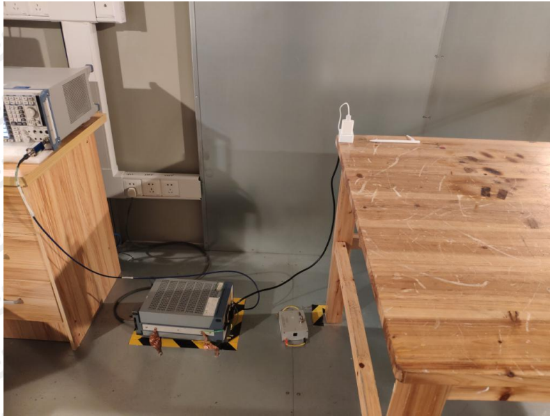
Photograph of test setup for Conducted Emission
